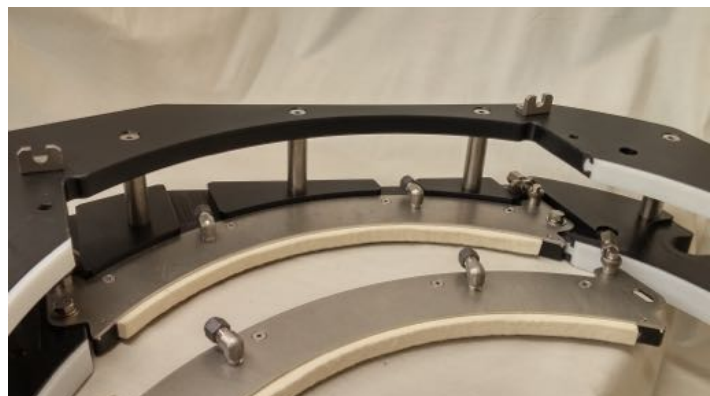
Image 2: Lower modular applicator pad installed. Adjusters on each pad control wax flow and even application around the bottle as it passes through.
