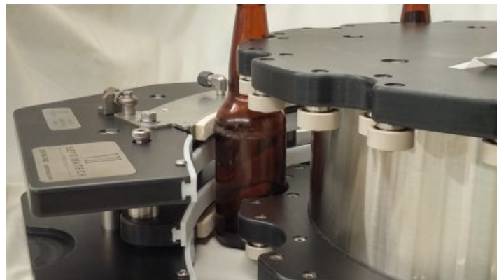
Image 4: Applicators installed in contact with the bottle.
