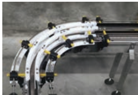
Adjust up to 80 feet of curved guide rails from one location in seconds, including curves, corners, crossovers and straight sections.
