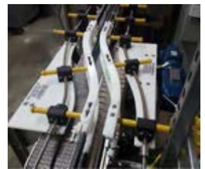
Adjust up to 80 feet of curved guide rails from one location in seconds, including curves, corners, crossovers and straight sections.
