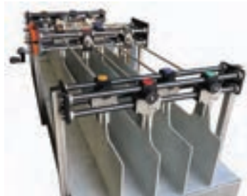
Easily create multiple lanes for different applications or products. Rapidly move unused lane dividers to conveyor outer edge when not in use.
