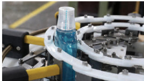
Superior container control in conveyor wheel corners.
