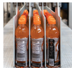
Easily create multiple lanes for different applications or products. Rapidly move unused lane dividers to conveyor outer edge when not in use.
